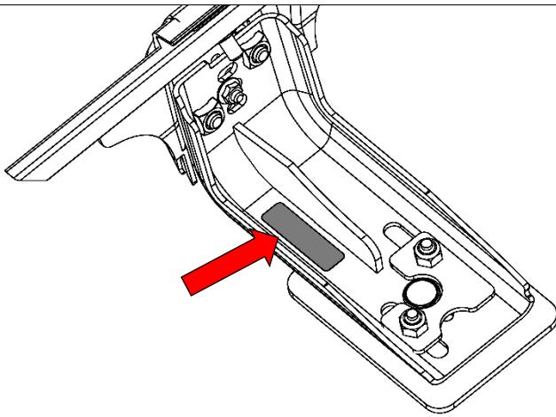
9. Place the compliance label on the rear driver's side leg in the location shown. Rub firmly to ensure adhesion.
