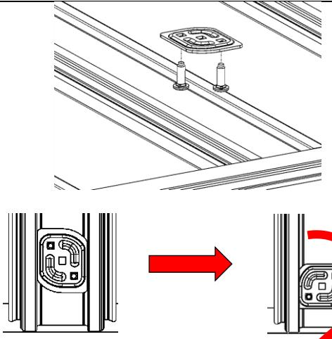
4. Insert the M8 studs into the stud plate
