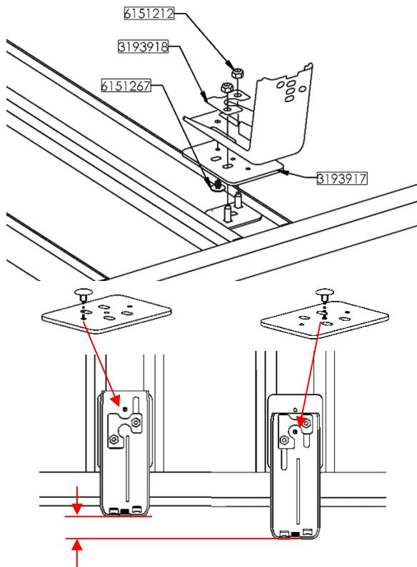
6. The support plate can be fitted in two positions depending on the width of the vehicle
